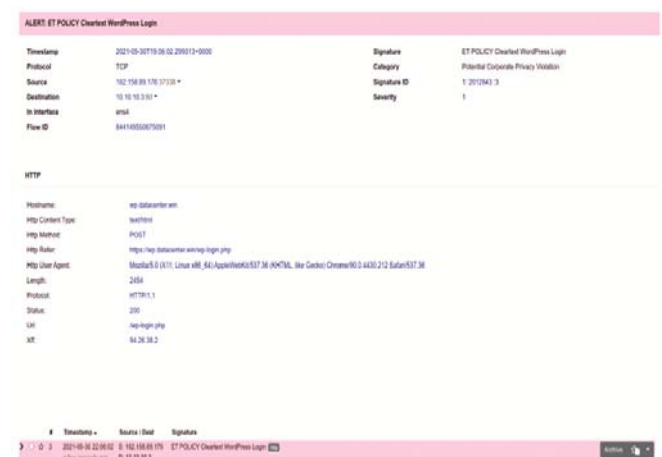
Fig. 3. Information from Suricata about detected vulnerability
