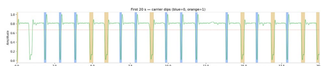
Fig. 5 DCF77 Carrier Dips — First 20 Seconds.
